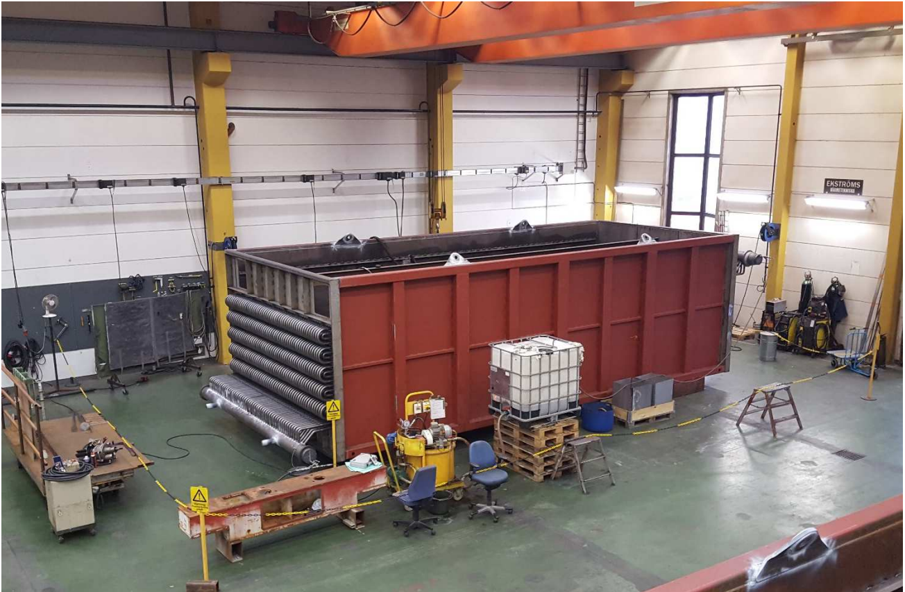
Economiser unit ready for hydro test in workshop, test pressure approx. 400 bar.
