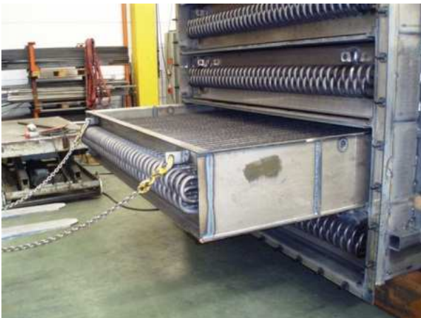
The Air preheater can be made as easily replaceable sections.
