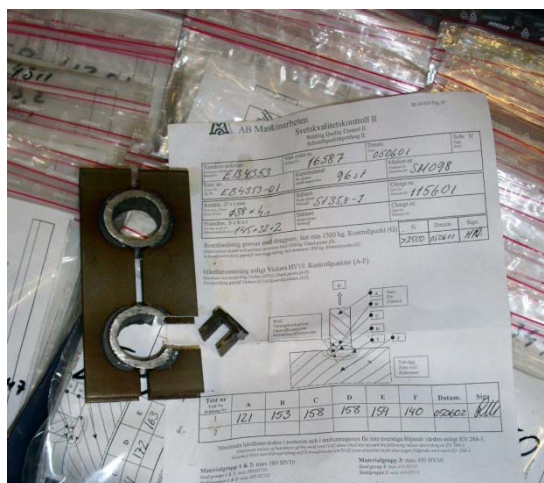
Control of fin attachment, hardness, dimensions etc. is made for every delivery of fin tubes.
